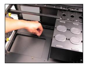
**Caution:** Make sure to remove any **unused** motherboard standoffs. They may come into contact with the back of the motherboard and may electrify your chassis exterior if left connected.
